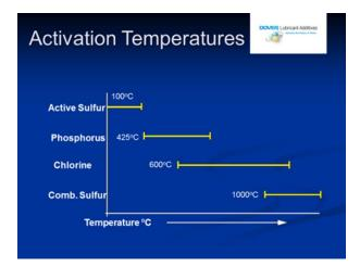
Take the example of active sulfur. One may place a drop of an active sulfur-containing additive, such as MAYCO BASE 1540, on a polished copper rod setting on a lab bench. Return a few hours later and notice the black stain. This is the reason active sulfur is not used on nonferrous alloys.
